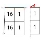
Bindery signatures are assembled with the closed edge on the same side and bound along a common edge
