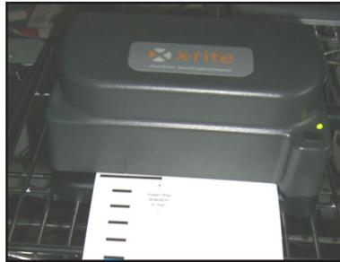
The unit will blink orange then green when it finishes calibrating. The window says the calibration is good for 18 hours. Close the calibration window. Return the DTP41 calibration strip to its envelope and store it in a safe place.
